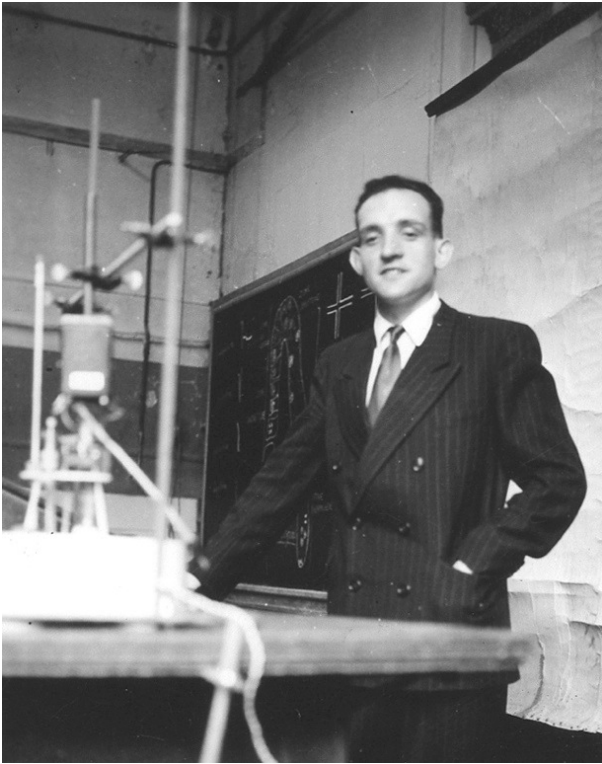
Figure 22. Jean Brun next to a highly precise temperature incubator for C. elegans cultures (PhD defense, 1966). The temperature-control system on the left was usually further placed in a temperature-controlled incubator with cooling, at a temperature of 22°C. Note the drawing of the C. elegans hermaphrodite gonad and meiosis on the blackboard. Courtesy of G. Brun.
